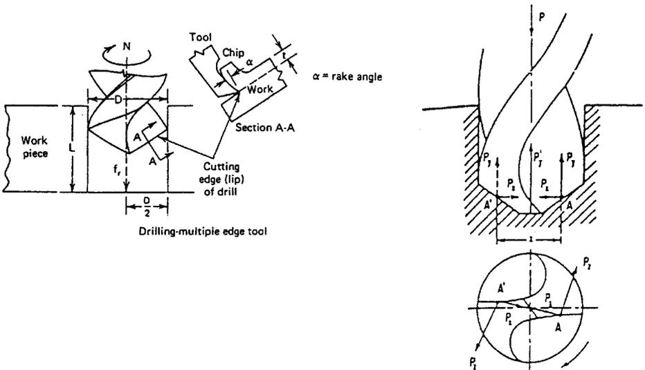
Fig. 33.14 Thrust forces and torque in drilling operation.
