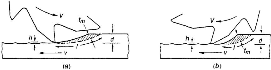
Fig. 33.19 Cutting action in up-and-down milling.
