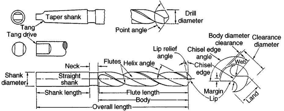
Fig. 33.13 Drill geometry.
