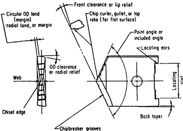
**Fig. 33.17** Spade-drill blade elements.
