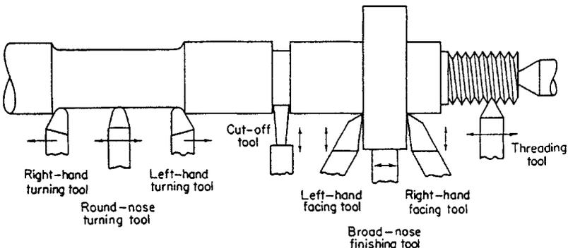
Fig. 33.9 Common lathe operations.
