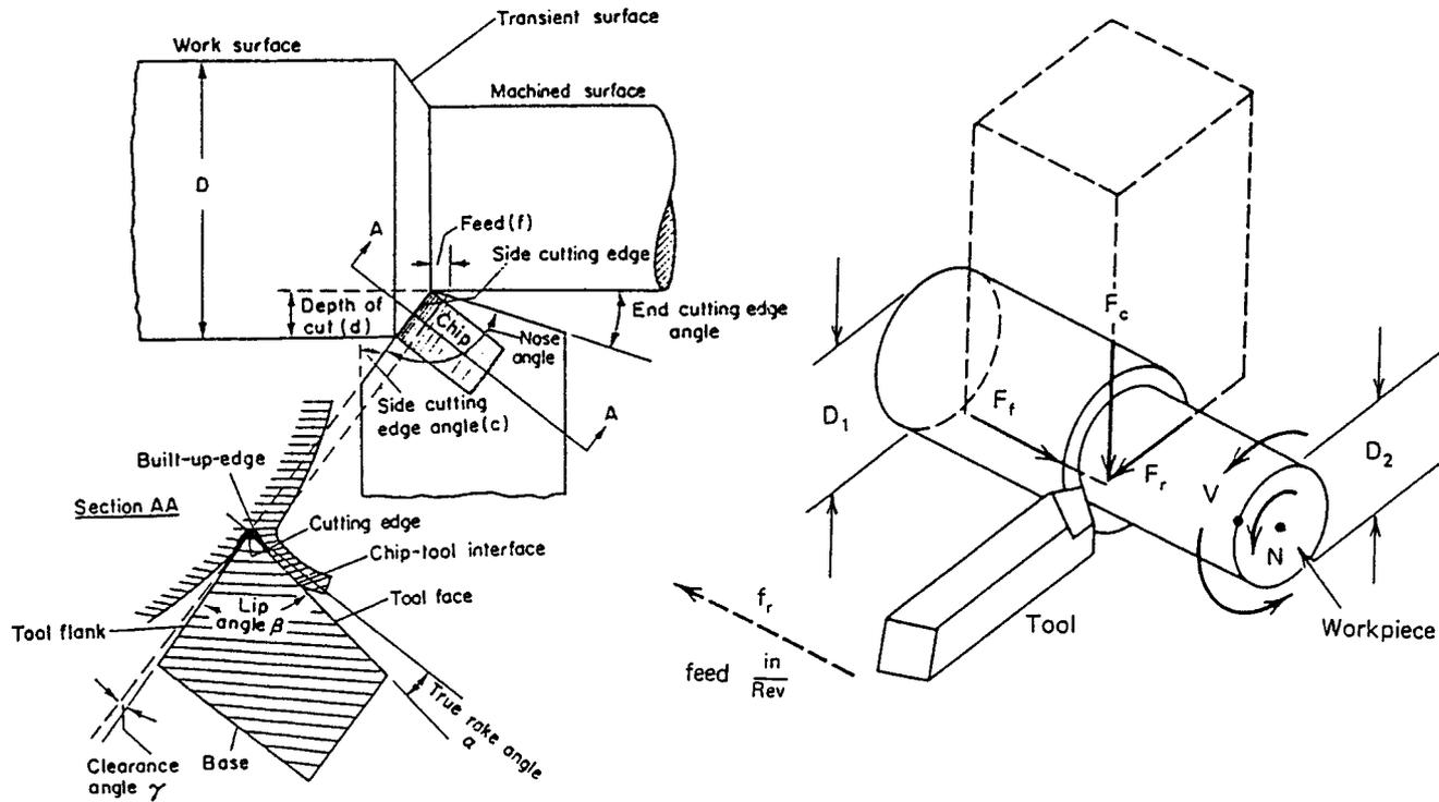
Fig. 33.10 Tool geometry—external turning.
