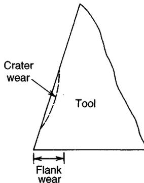
**Fig. 33.5** Types of tool wear.
