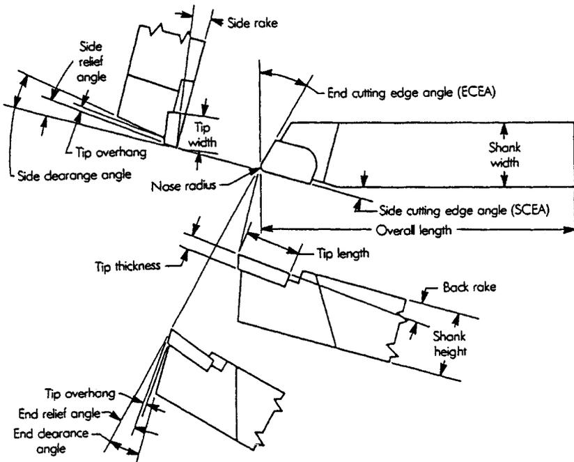
Fig. 33.8 Basic tool geometry.
