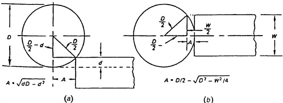
Fig. 33.20 Allowance for approach in (a) plain or slot milling; (b) face milling.
